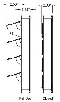
\* W & H dimensions are approximately 1/4" undersized. Box Frame shown above, Flange will add 1-1/2" around perimeter
